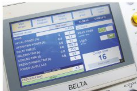
Touch screen HMI/PLC, cycle memory and ATS™ power control
