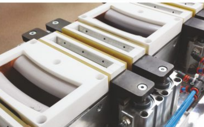
Belt edge stops and pneumatic belt holders
